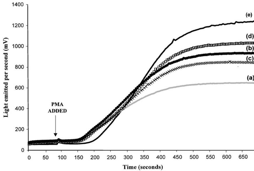
Fig. 3. Plots of light output (mV) versus time (s) for heparinised diluted blood (1:100) that has been exposed to (a) HA, (b) HA heated to 800°C (c) HA(MW) (d) HA(MW) heated to 800°C and (e) the corresponding PBS control.
