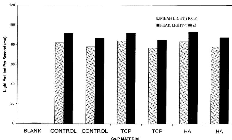
Fig. 7. Histogram of the mean and peak light output (mV) measured over 100 s from solutions containing Pholasin<sup>®</sup> and PMA only (no blood) in contact with as received TCP and HA. Data from the corresponding controls are also shown.
