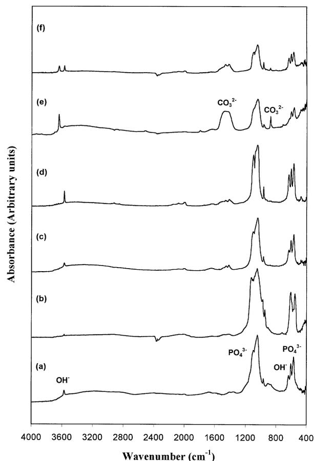
Fig. 5. FTIR spectra (4000–400  $\text{cm}^{-1}$ ) for (a) TCP, (b) TCP heated to 800°C, (c) HA, (d) HA heated to 800°C, (e) HA(MW) and (f) HA(MW) heated to 800°C.
