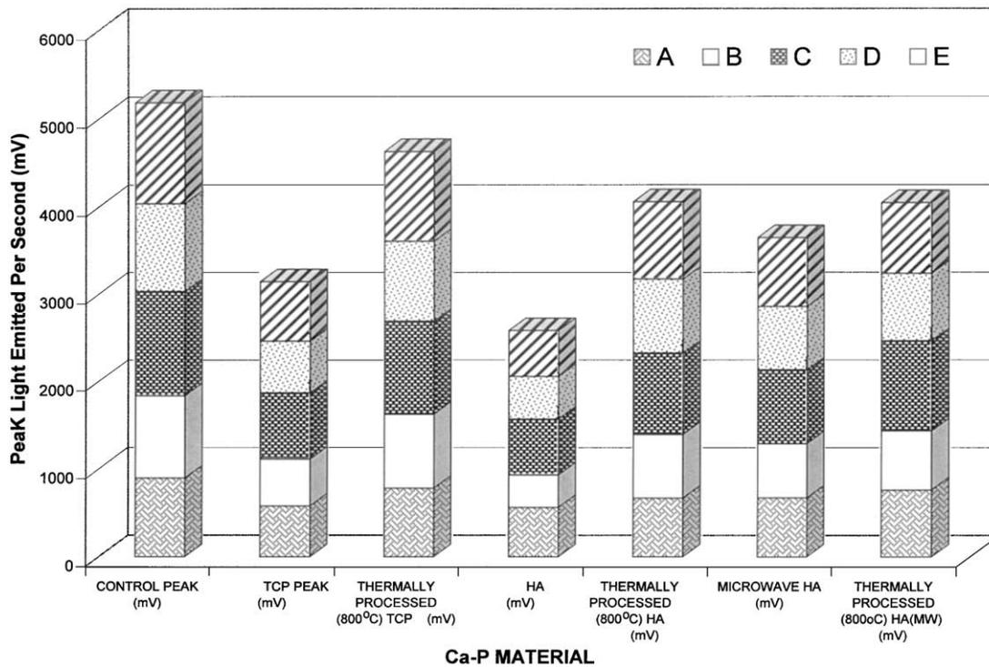
Fig. 4. Histogram of peak light emission per second (mV) for the six Ca-P materials (as received and heated 800°C) obtained after exposure to heparinised diluted blood (1:100) from each of the five blood donor samples.
