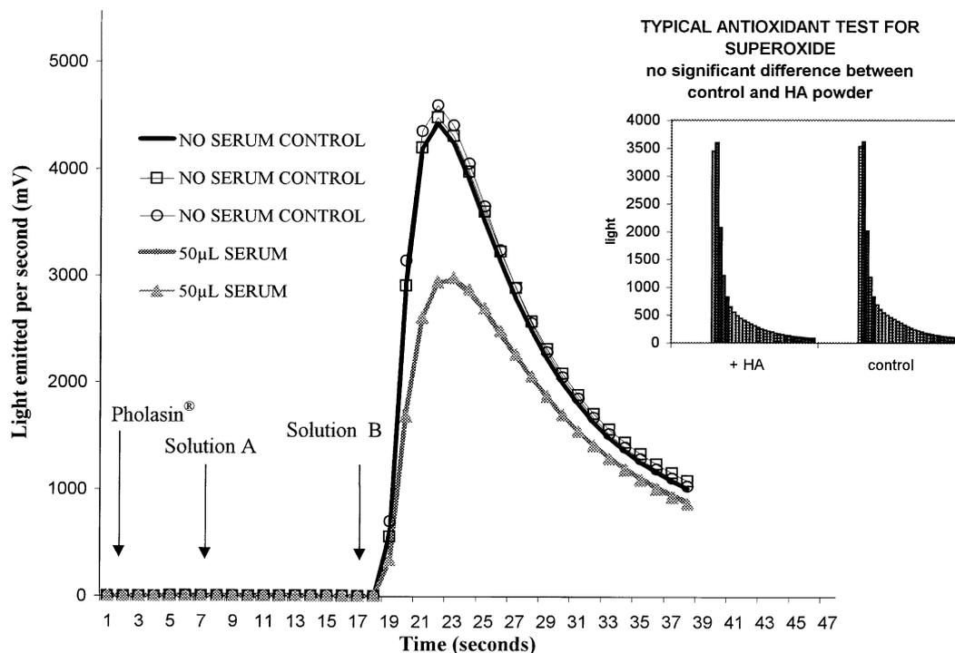
Fig. 8. Plots of light output (mV) versus time (s) illustrating a 44% reduction in luminescence caused by competition for superoxide by addition of serum. Insert shows no significant reduction in light output caused by exposure to HA compared to that from the corresponding PBS control.
